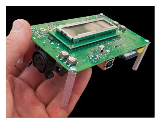
Another option is to run complete shows on a scheduled basis using a completely solid-state standalone playback device. In addition to DMX output, it has a serial port for output, another for control, plus an IR remote control. It output stereo audio and features an SD slot for unlimited show and audio capacity.
